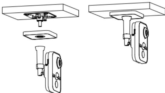
**Figure 3-8 Install the Camera**
