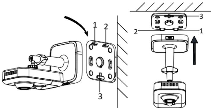
Figure 3-11 Buckle the Camera into Adapter Plate
