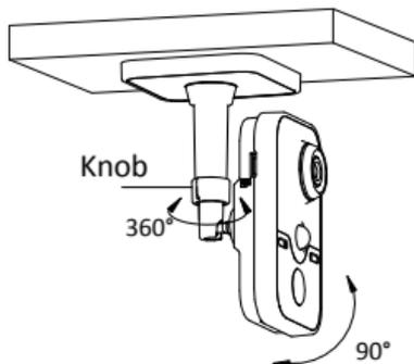
Figure 3-9 Adjust the Camera
