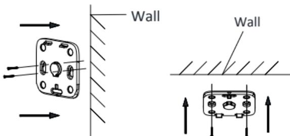
Figure 3-10 Install the Adapter Plate
