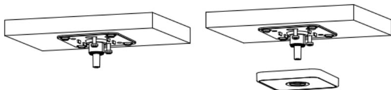
**Figure 3-7 Install the Fixed Plate and Mounting Base**
