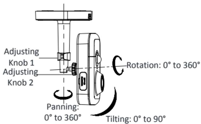
Figure 3-12 Adjust the Camera
