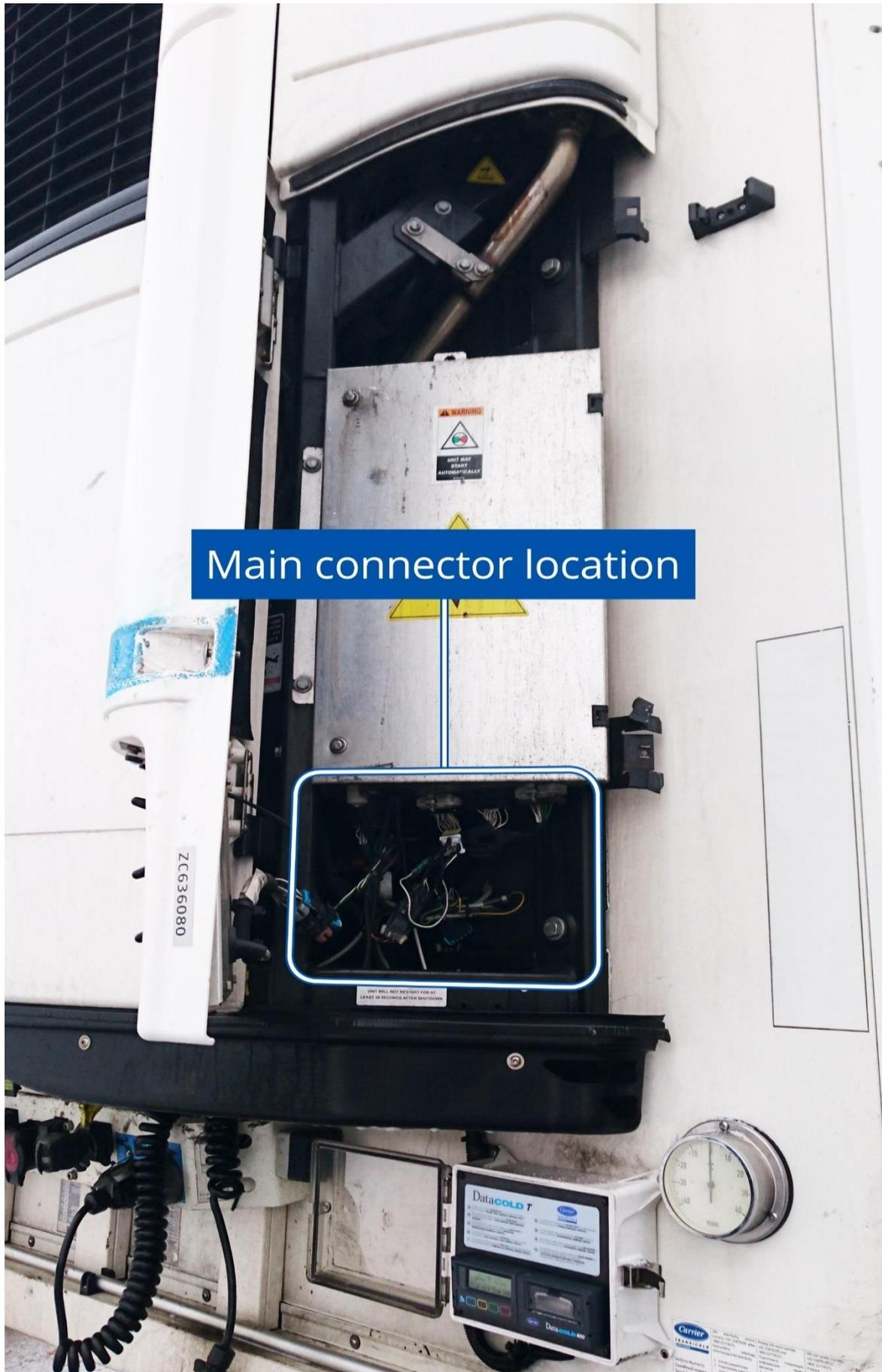
Figure 4 The main connector location
