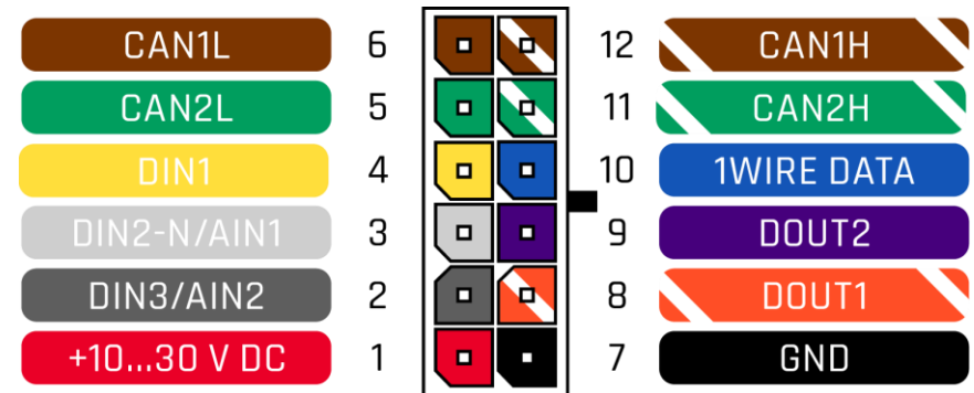
Figure 2 FMB140 2x6 socket pinout
