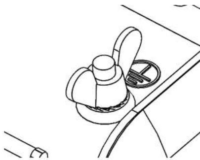
The device includes a grounding connection (marked  $\equiv$ ).
