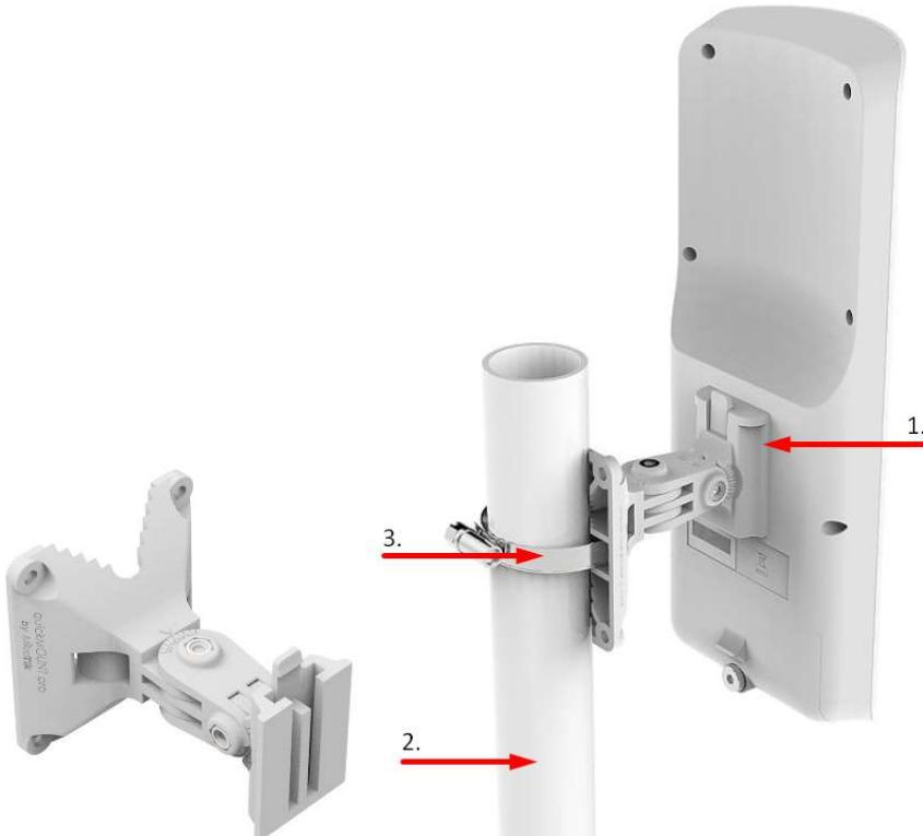
2. Attach the device to the pole.
