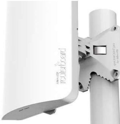
4. Please avoid connecting a loose Ethernet cable to the Ethernet port, secure the cable to a wall or the pole, so that the cable weight is not pulling the port. It is recommended to secure the Ethernet cable less than 2m from the device. This is to ensure that the cable doesn't damage the port by its weight, or doesn't fall out.
